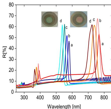
**Figure 2:** Reflectance spectra of two sets of NAA samples (green and red range) for different pore diameters: a) 38 nm, b) 42 nm, c) 46 nm and d) 50 nm. Inset: digital images of the NAA samples.
