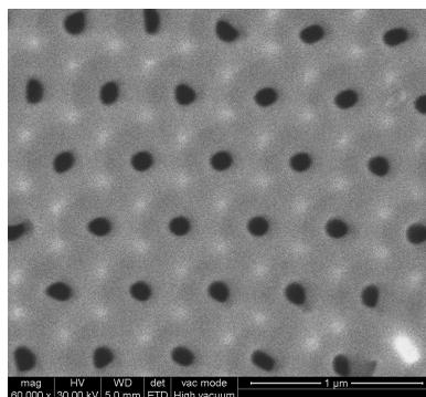
**Figure 1:** Example of top view SEM image of self-ordered nanoporous anodic alumina. The pore diameter is 95 nm.
