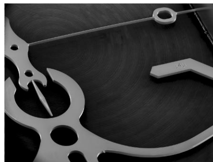
Figure 2. Constant escapement spring structure by Girard Perregaux. The width of the bi-stable spring is 14 microns for a thickness of 120 microns and a length of 2 cm.
