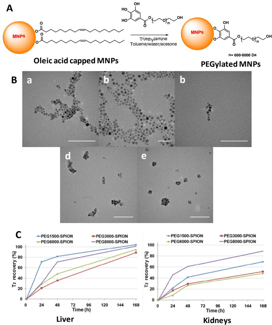
**Figure 1.** A) Scheme of ligand exchange procedure.; B) Representative TEM images of water soluble molecular weight PEGylated iron oxide nanoparticles: a) PEG600-SPIONs; b) PEG1500-SPIONs; c) PEG3000-SPION; d) PEG6000-SPIONs and e) PEG8000-SPIONs. Scale bar corresponds to 50 nm. And C) T<sub>2</sub> recovery of the liver and kidneys after PEG-MNPs injections.
