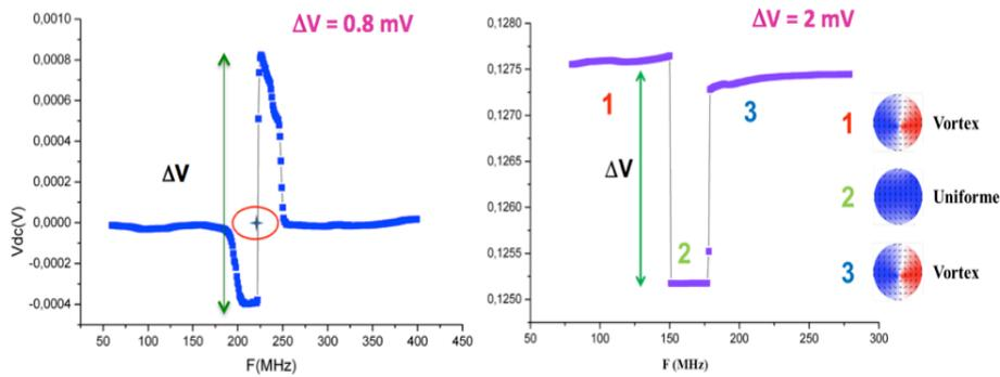
Figure 1. a) Rectification effect detected for a STNO with one vortex, of diameter  $D = 400$  nm at  $I_{DC} = 0$  mA,  $P_{RF} = -4$  dBm and  $H = -1700$  Oe b) Vortex core expulsion detected for a STNO of diameter  $D = 500$  nm at  $I_{DC} = 6$  mA,  $P_{RF} = -4$  dBm and  $H = -2000$  Oe
