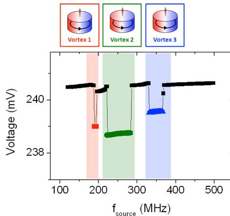
Figure 2. Three vortex core expulsions for three STNOs with one vortex, of diameter  $D = 500$  nm (red), 400 nm (green) and 300 nm (blue).
