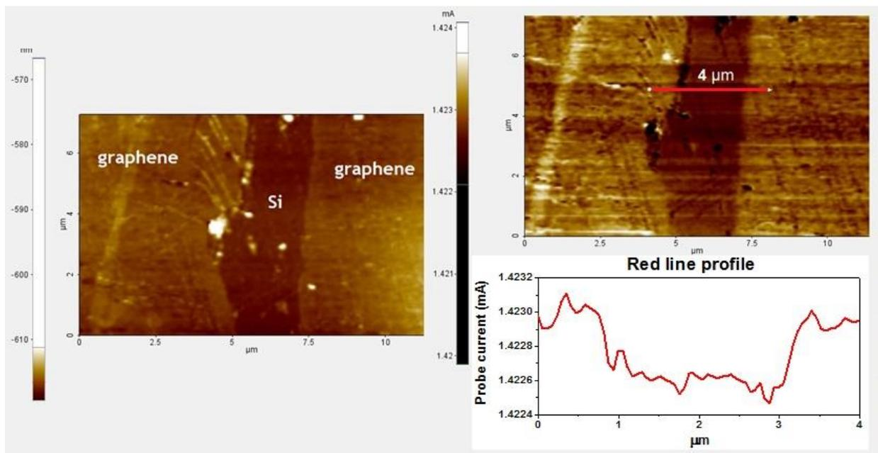
Fig. 2 Left: topographical image of Si/graphene interfaces performed with thermal nanoprobe of SThM system; Right: SThM conductivity contrast image (CCM) of the area depicted on the left and line profile showing the contrast in thermal conductivity between graphene and Si
