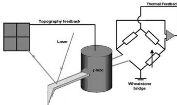
Fig. 1 Schematic showing the independent nature of both mechanisms for topographical and thermal images collection (adapted from Park Systems [2])
