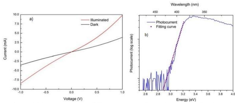
Figure 2: a) I-V curve and b) PC spectrum of graphene / ZnO photodetector.
