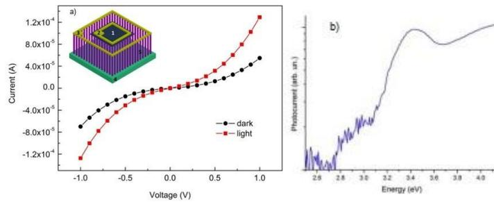
Figure 3: a) I-V curve and b) PC spectrum of graphene / GaN photodetector. The inset of Fig a) shows the photodetector schematic.
