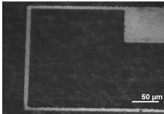
Figure 1: processed graphene / ZnO NW photodetector.
