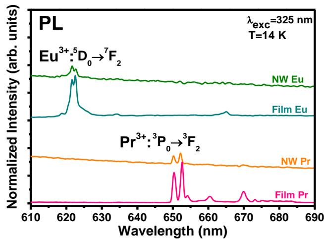
Figure 1 - Comparison between the PL emission of the GaN NWs doped with  $\text{Eu}^{3+}$  and  $\text{Pr}^{3+}$  ions and the GaN films doped with the same ions.
