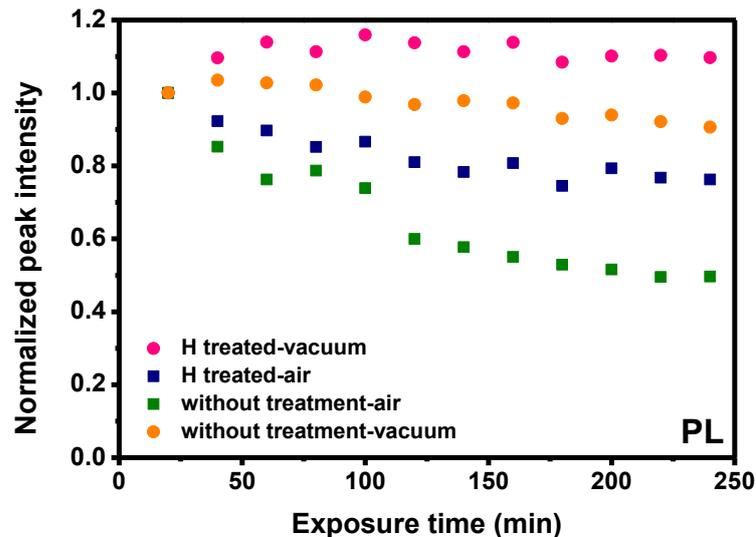
Figure 2 - Maximum peak intensity of the yellow band for the annealed GaN:Er NWs before and after the treatment with H plasma, as a function of the He-Cd laser exposure time. The data are normalized to the maximum of first spectrum (20 min) for each ambient.
