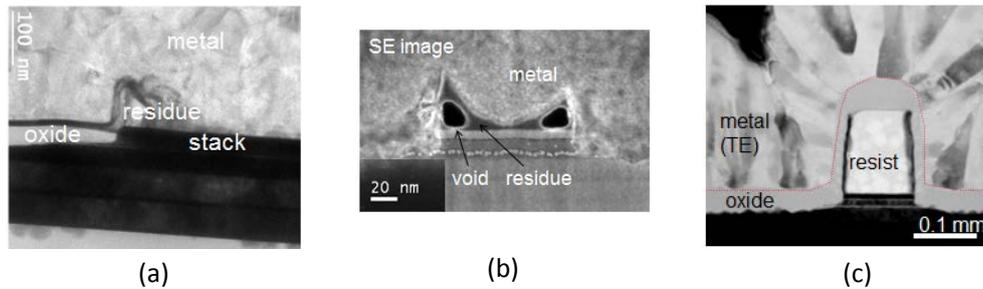
Fig. 1: (a) Nanopillar with lift-off residue along the pillars boundary; (b) Nanodevice with voids in TE, lift-off-based process failed [5]; (c) Nanodevice with resist buried inside oxide lag [5].
