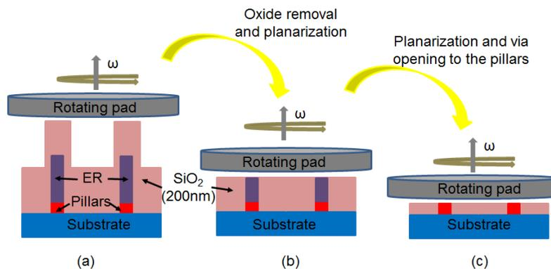
Fig. 2: The schematic diagram of CMP-based nano-fabrication process.
