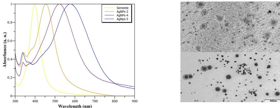
Figure 1. (left) Normalized absorption spectra for silver colloids; (yellow) seeds, AgNPs-1; (orange) AgNPs-2; (purple) AgNPs-4 and; (blue) AgNPs-5. (right) TEM image for AgNPs-5 sample.
