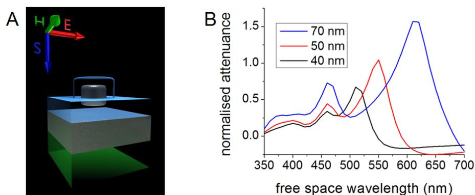
**Figure 1.** **A)** Single cell of a periodic array with single cylinder and silver layer. Materials: silver (grey), alumina (blue) and fused silica (green). **B)** Example of normalized attenuation (reference subtracted) for structures with an underlying silver layer.
