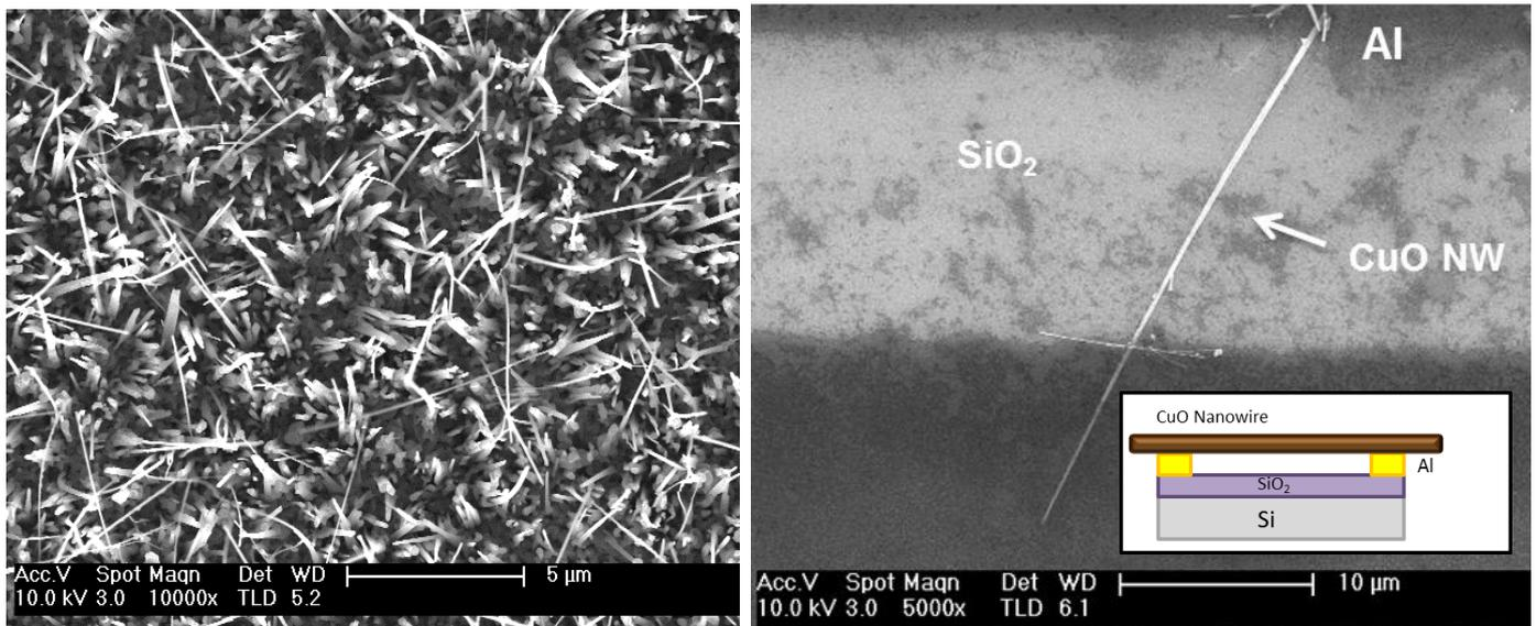
Fig. 1: Scanning electron microscope images: CuO nanowires thermally grown (left) and CuO NW dielectrophoretically aligned (right).
