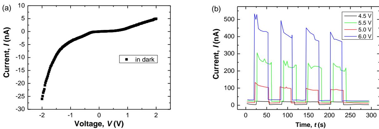
Fig. 2: Current-voltage curve for CuO NWs in dark (a) and their response to a halogen lamp (b).
